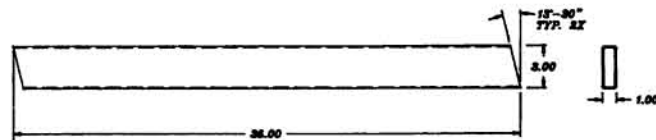
8 MAT'L. TUBE 1 X 3 X .094 WALL EW STEEL 2 REQ'D.
